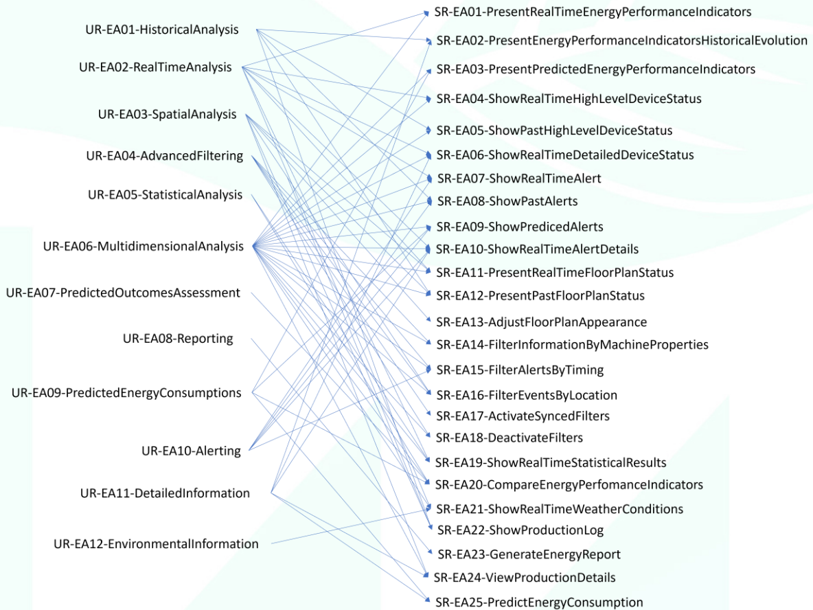
Figure 34 The mapping of the user requirements related to energy analysis to the relevant system requirements
