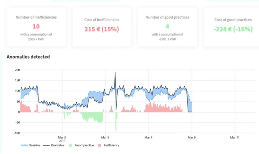
Figure 19 EMS functionalities: a) Alerting (anomaly detection)
