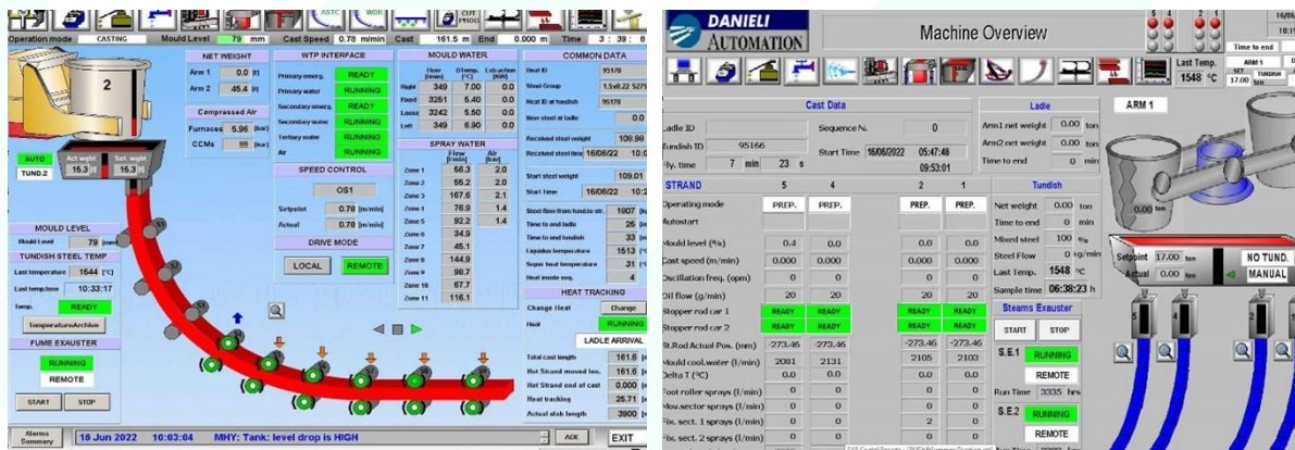
Figure 11 Monitoring the casting temperature
