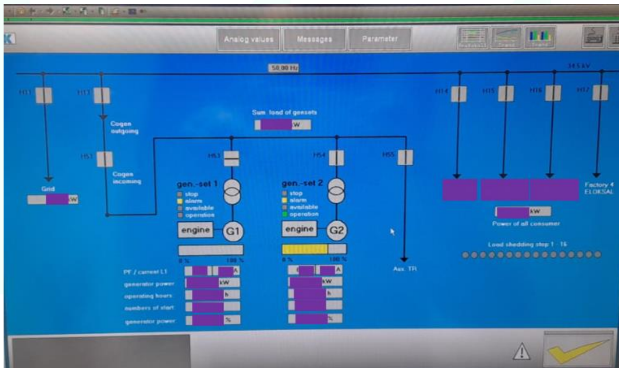
Figure 1 Current visualisation of electricity generation monitoring for ASAS (sensitive information is hidden)
