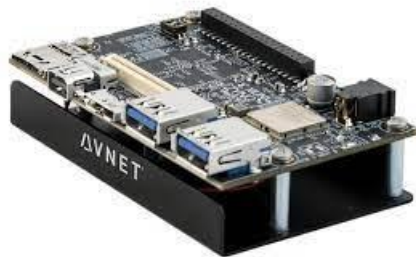
Figure 24. The ULTRA96 Board that is used in this Demo
